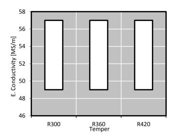
Electrical conductivity is strongly influenced by chemical composition. A high level of cold deformation and small grain size decrease the electrical conductivity moderately. Minimum conductivity level can be specified.
