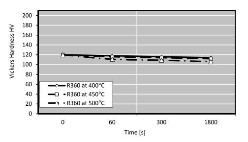
After short time heat treatment Vickers Hardness is measured. The diagram shows typical values.
