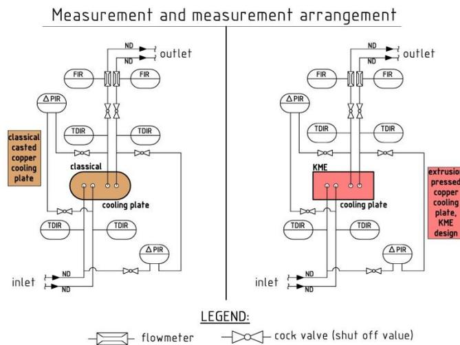
Fig. 6: Scheme of Copper Plate Cooler experimental equipment at site
