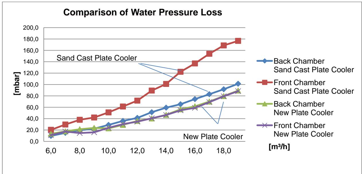
Fig. 12 Comparison of water flow and pressure loss for the sandcasted and new Copper Plate Cooler
