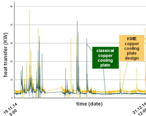
Fig. 9: Heat Transfer Comparison of two Different Copper Plate Cooler Designs
