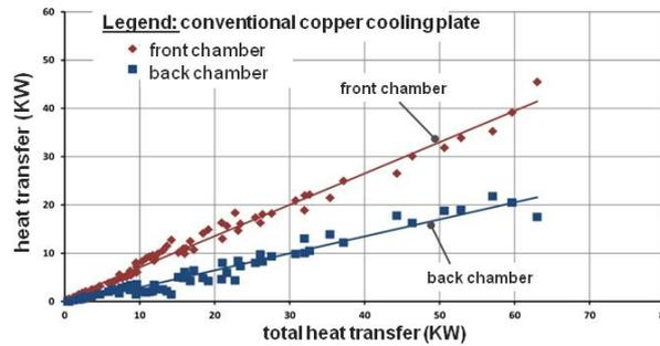
Fig. 10: Total heat transfer measurement of the sandcasted copper Plate Cooler
