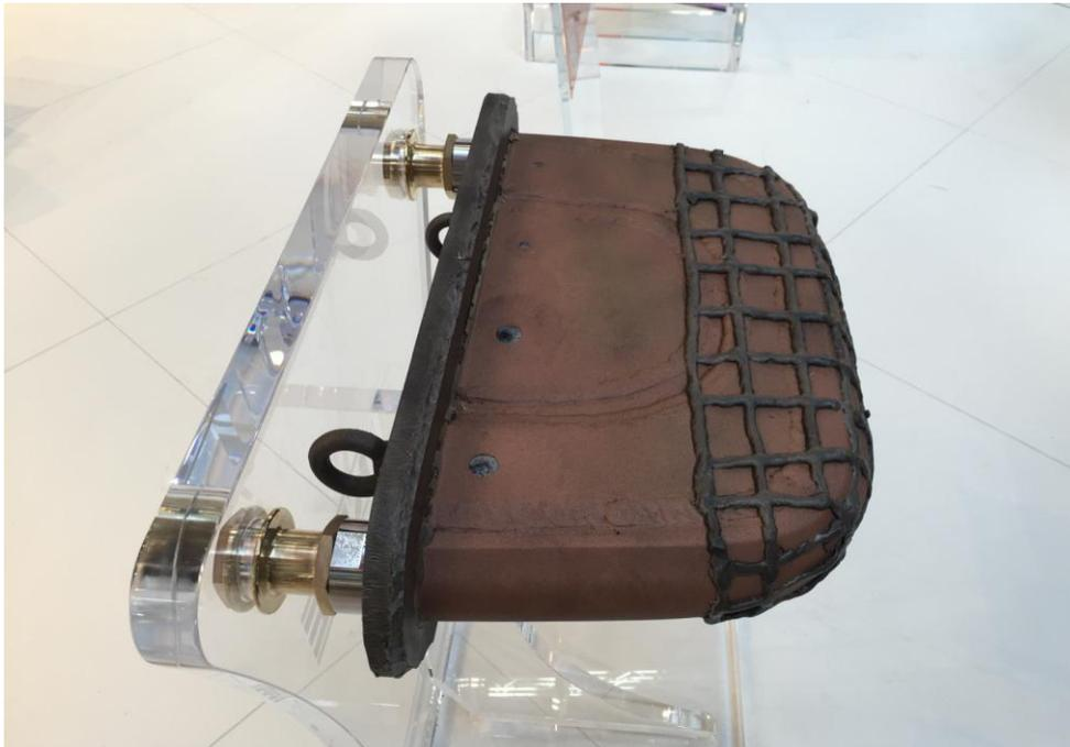
Fig. 0: KME Copper Plate Cooler
