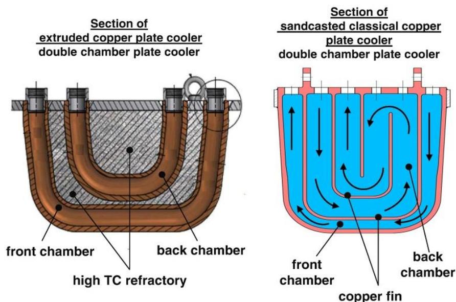
Fig. 3: Comparison of the two different copper Plate Cooler designs
