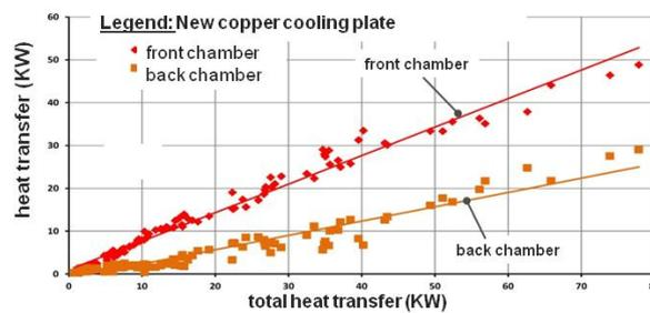
Fig. 11: Total heat transfer measurement of the new copper Plate Cooler
