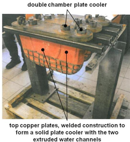
*Fig. 4: New Copper Plate Cooler Design*
