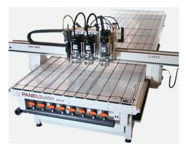
Fig. CNC machining centre, Panel Builder, from AXYZ International
