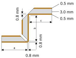
Fig. in- and exterior corner 90°
