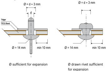
Connection of two or more metal parts joined together, drilled, and pierced by a rivet.
