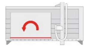
It is advised to use guide rails, which overlap the panel ends a minimum of 200 mm. Multiple panels can be cut simultaneously.
