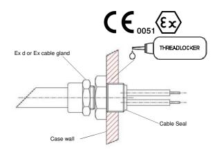
Proceed as follows to complete the termination. Screw the self threaded brass pot on the cable sheath, placing the inner part of the hole on the copper sheath.
