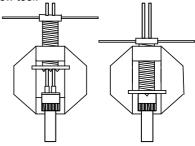
Cut some lengths of sleeving and, after removing eventual exceeding sealant, place them on the stub cap.
