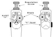
Start rotating the tool pushing it towards the inner part of the cable; avoid the rolling up of the copper shaving on the conductors, fixing it on the suitable hook.
