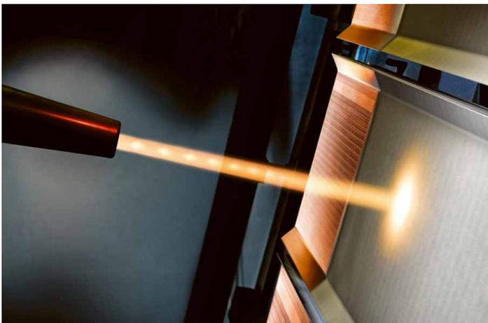
As there is little difference between the thermal characteristics of standard nickel and AMC®-HN 40 coatings there is no need to adapt the cooling and casting parameters when using AMC®-HN 40. Both types of coating can be applied in greater thickness so that they can be remachined several times.
