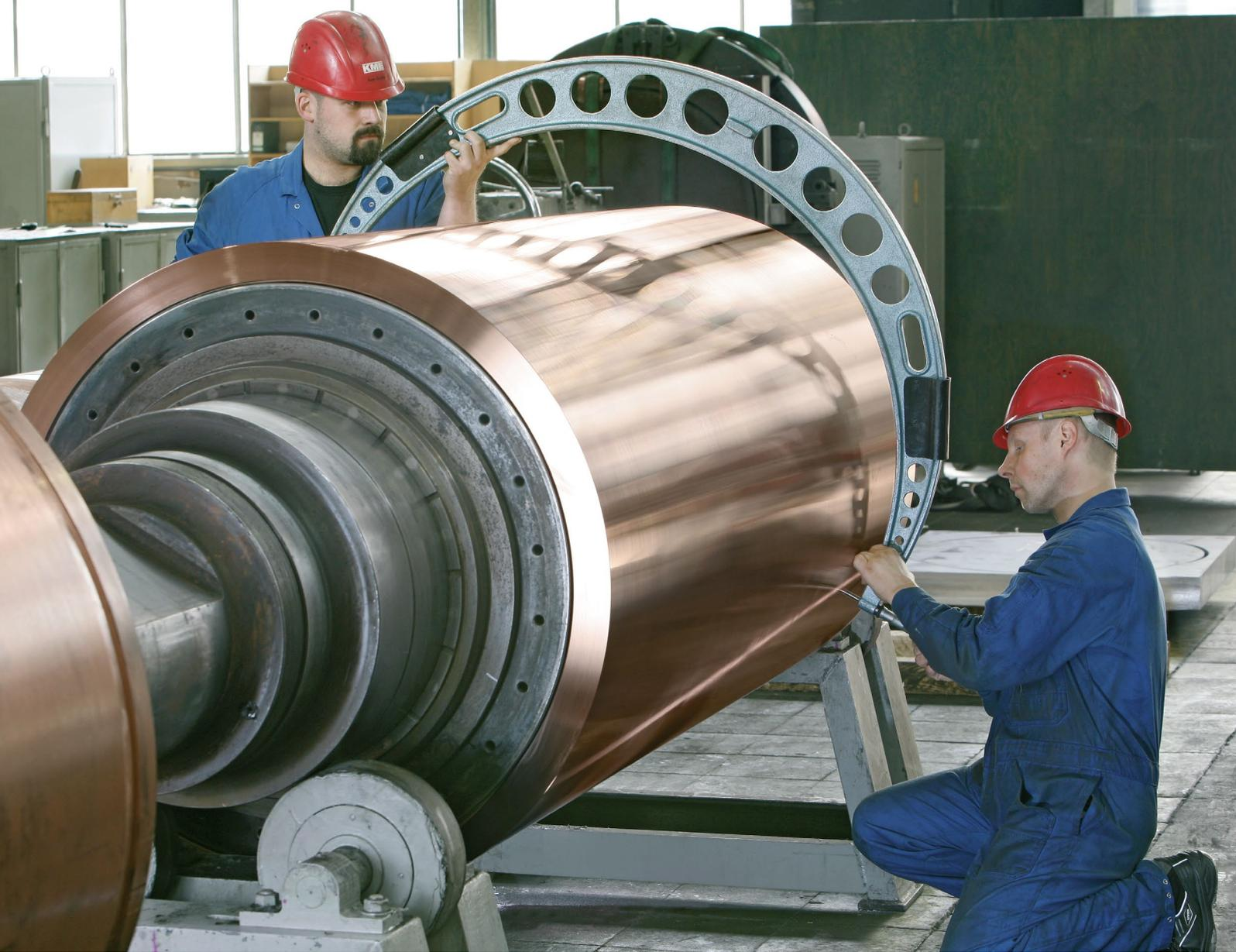
Against this background KME started the development of copper alloys suitable for sleeves for aluminium strip casting.
