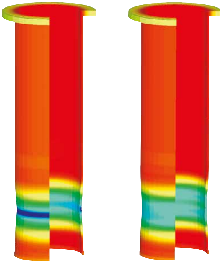
FEM simulation of the distortion of a crucible during cyclic thermal stress for different materials
